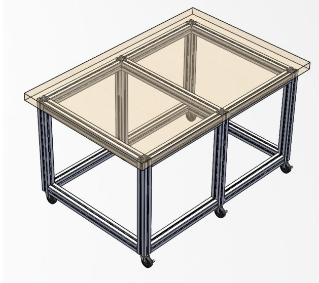
Figure 6.9 3D model of the testbench (appearance of the wood countertop set to be transparent)
