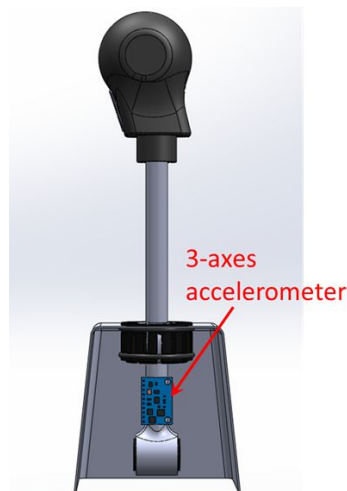
Figure 6.6 3D model of the gear lever and the sensor
