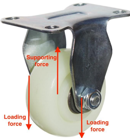
Figure 6.3 Schematic representation of force analysis for the shaft of roller
